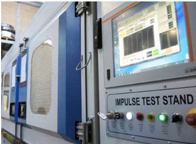
Banco per prova ad impulsi secondo norma SAE Bench for impulse pressure test according to SAE standard
