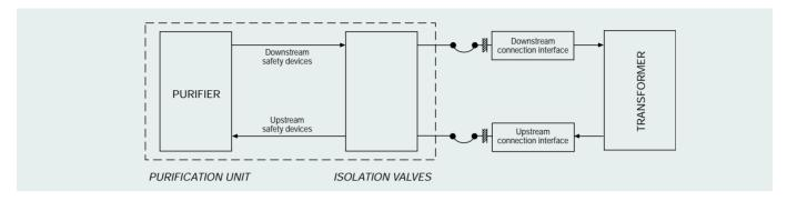
In order to carry out the transformer treatment under load in complete safety, the purifying installation comprises the following elements:
