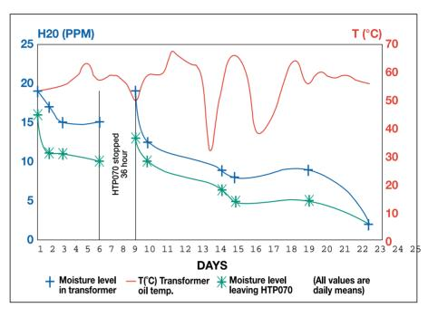
The above example shows the treatment of a transformer of 23 MVA containing 8.5 tonnes of oil. The water content before treatment was 30 ppm at 20°C and the water content several months after the treatment remained at 6 ppm at 20°C.
