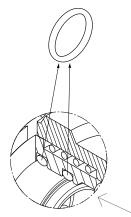
Push the bushing to replace the O-Ring
