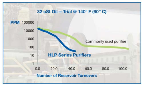
HLP Series oil purifiers showed a 40% faster dehydration rate when compared with a typical purifier.
