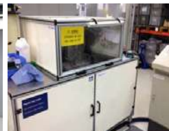
Impulse pressure test stand up to 4000 bar.
