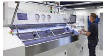
Flow test stands for hydraulic oil and water, capacity up to 300 l/min.
